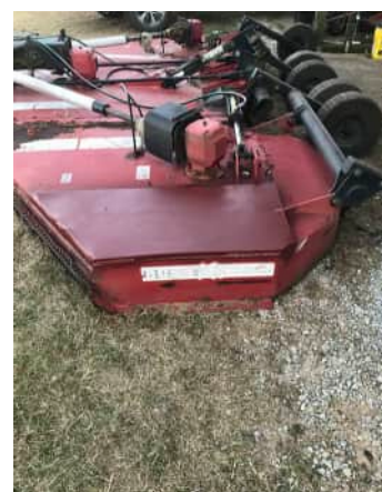
Repaired the plant Bushhog by welding new structural supports for the gear box and surface plates.
