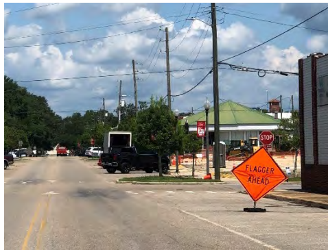
Example of a stop sign that is difficult to see due to its position at the intersection, particularly if cars are parked on street.
